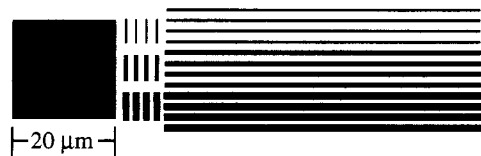
Figure 2. Electron-beam exposure pattern. The pattern was either a series of single-scan, 0.1- and 0.2- \mu\text{m} linewidths with 1.8-, 1.7-, and 1.6- \mu\text{m} spaces or a series of single-scan, 0.3- and 0.5- \mu\text{m} linewidths with 1.8-, 1.5-, and 1.3- \mu\text{m} spaces.
